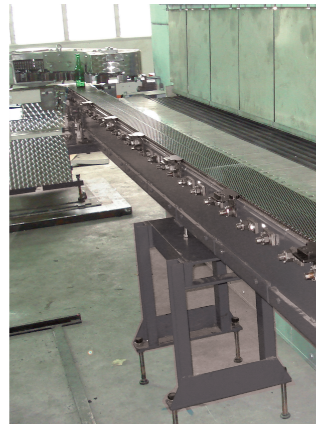
Return head Special execution, with use of a Pennekamp ware transfer
