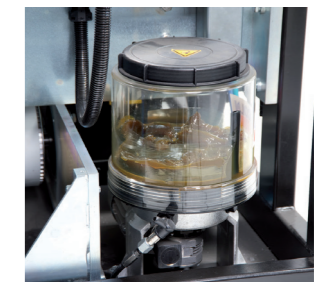
Automatic lubrication system for maintenance free operation
