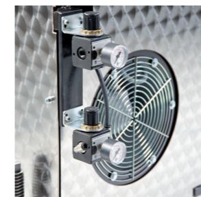
Pressure fan for machine cooling
